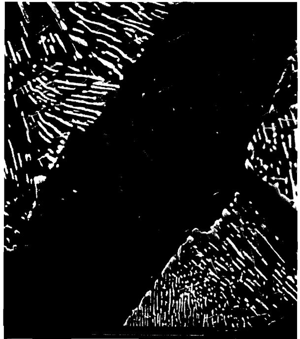
Plate 3: 1.55 SEM photomicrograph (3000 \times ) showing nitride needles in ferrite surrounded by partially spheroidized pearlite.
