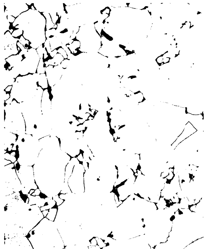
Plate 4: I.77 Photomicrograph (400X) of zone of large ferrite grains showing minimal evidence of carburization.
